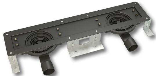
6. Connect the trap[s] to the waste pipe. Mask the top of the drain to prevent debris entering the trap when the screed is laid.
