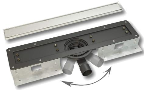
3. When the drain is in the correct position secure the legs to the sub-floor with appropriate fixings. Use the additional rear fixing brackets to secure the legs closest to the wall. Set aside the stainless steel grill and frame for later use.
