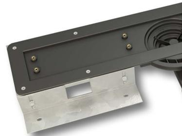
4. Loosen the 8 bolts and set the height of the drain approximately 12-15mm lower than the height of the screed to allow for a fall to be created when the screed is laid.
