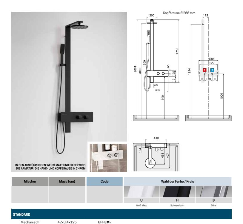
**DURCHMESSER KOPFBRUASE 20CM BEI 3 BAR WASSERDRUCK** 15 L/MIN BEI DER KOPFBRAUSE **7 L/MIN BEI DER HANDBRAUSE**
